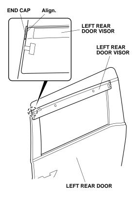
19. While applying light pressure against the left rear door visor, carefully remove the adhesive backings. Push up on the rear brackets while removing the adhesive backings.
