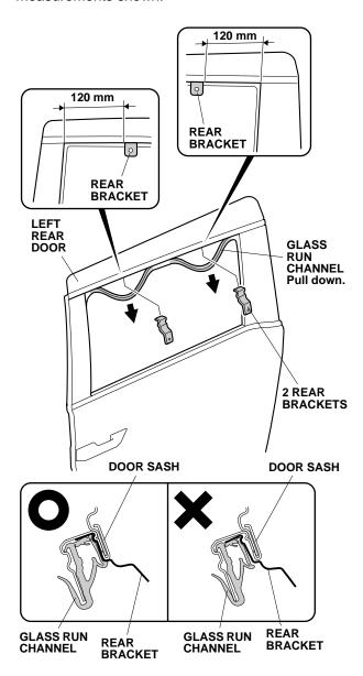
13. Reinstall the glass run channel to secure the two rear brackets. Be sure the brackets are installed tightly to the door sash, and that the glass run channel is properly seated. 14. Using isopropyl alcohol on a shop towel, thoroughly clean the door where the left rear door visor will attach.
