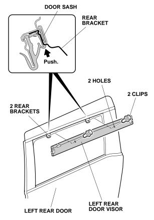
17. Secure the left rear door visor to the front brackets with two clips. Push up on the rear brackets while installing the two clips. Install the clips correctly, they cannot be removed. 18. Adjust the position of the left rear door visor as shown.
